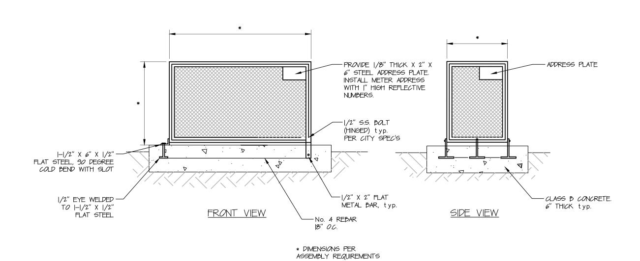
— NATIONAL MFG. CO. # V6, STK. #100-313 EXTRA HEAVY PULL, WELDED TO FRAME. FLAT BAR SUPPORT, — CENTER AT TOP, typ. 44 4 4 4 -GRATING: 3/4" #9 FLAT EXPANDED METAL, WELDED TO CORNERS, 4 4 4 4 4 4 4  $|-|/2" \times |/2"$  FLAT STEEL - WITH SLOT TO ACCOMMODATE TOP VIEW --- |--|/2" x |--|/2" x |/8" ANGLE IRON FRAME WITH BUTT WELDED, MITERED CORNERS, 1/2" EYE \* DIMENSIONS PER ASSEMBLY REQUIREMENTS
