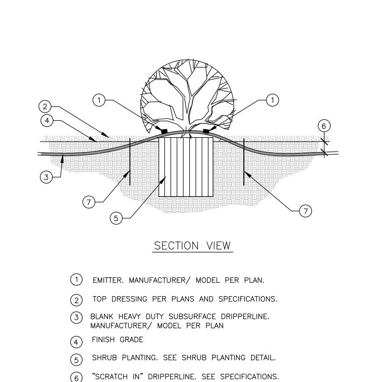
7 METAL SOIL STAPLE. 6" MINIMUM LENGTH @ 4'-0" O.C., AT CHANGES IN DIRECTION, AND AT FITTINGS.
