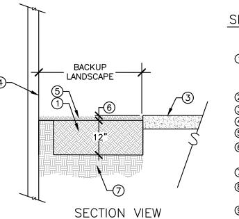
(1) RIP PLANTER SOIL IN PLACE TO DECOMPACT. 30" MINIMUM DEPTH AT MEDIAN, 12 MINIMUM DEPTH AT BACKUP LANDSCAPE). LEAVE IN PLACE. COMPACT TO 85% RELATIVE DENSITY.
